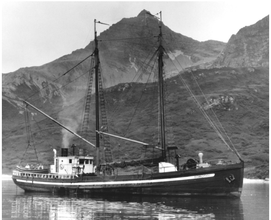
Figure 1.—The halibut schooner Dorothy , which participated in the 1940–41 Alaska king crab exploration and in the 1948 Pacific Explorer fleet expedition. Its small engine could be supplemented with sail supported by two masts. Bottom trawl gear was set and retrieved over the side. The dories on the stern of the vessel were used by pairs of men for halibut hand-lining. Photo of the Dorothy at Mitrofanina Island, Alaska, courtesy of the Lokken collection (#212012) at the Museum of History and Industry, Seattle, Wash. Photo credit: Puget Sound Maritime Historical Society.
