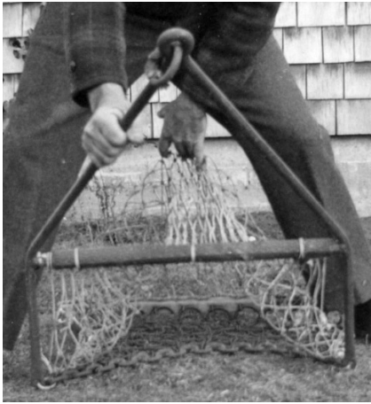
Figure 28.—A bay scallop dredge with linked chain on its leading edge at the bottom, Edgartown, Mass., about 1950.
