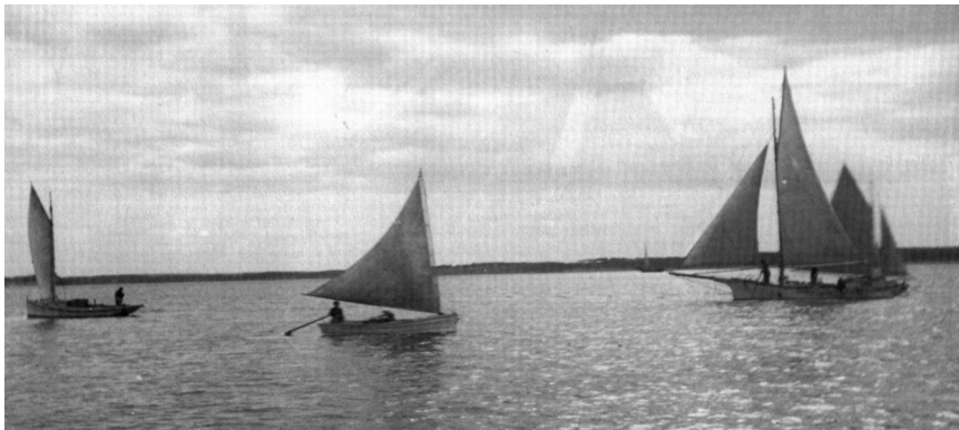
Figure 95.—Dredging for bay scallops in a light wind, Peconic Bay, N.Y., 1915. Shown are a catboat (left), sharpie (center), and three sloops (right). Source of photograph: Lightfoot et al., 1984.
