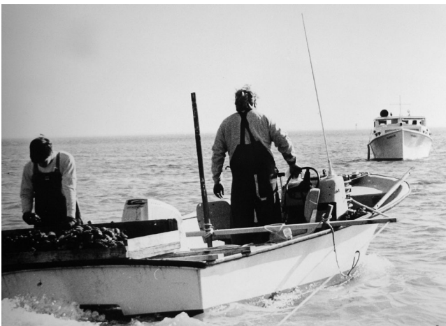
Figure 26.—The North Carolina scalloping boats have a pole across them to spread out the dredges they are towed. Photograph courtesy of North Carolina DMF.
