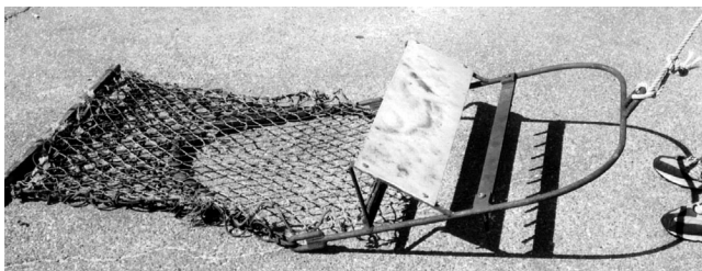
Figure 30.—A bay scallop dredge with pressure plate is termed a pan dredge, Westport, Mass., 2006.
