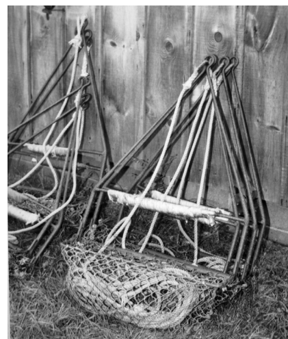
Figure 101.—Bay scallop dredges stacked alongside a former fisherman's garage, Flanders, Long Island, N.Y. Scallops were too scarce for harvesting in 2006 when this photograph was taken.
