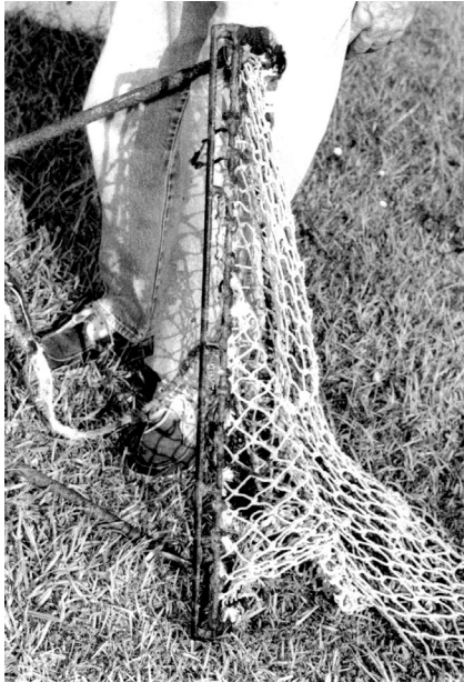
Figure 29.—A bay scallop dredge with bar on its leading edge at the bottom. Two parallel bars are used; the lower one scrapes along the bottom; the netting is attached to the upper one so it will not be worn by scraping against the bottom sediments.
