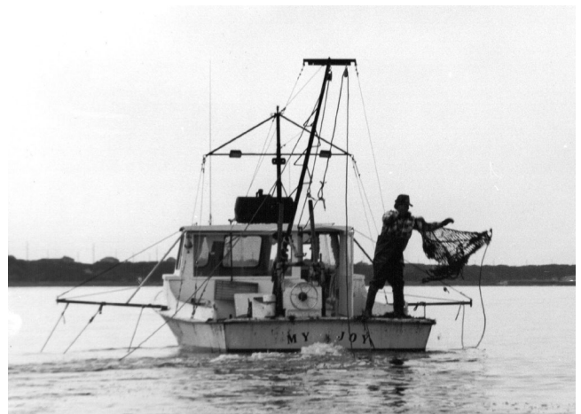
Figure 27.—This North Carolina boat tows eight dredges to harvest bay scallops; the poles extending from the hull spread out the dredges. Photograph courtesy of North Carolina DMF.
