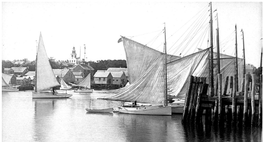
Figure 19.—The sails of catboats had to be raised for drying if they became wet, to prevent rotting, Nantucket, Mass., about 1920. Photograph courtesy of Nantucket Historical Society.
