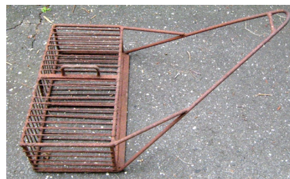
Figure 108.—The New Jersey bay scallop dredges were constructed entirely of iron and had a rigid bag.
