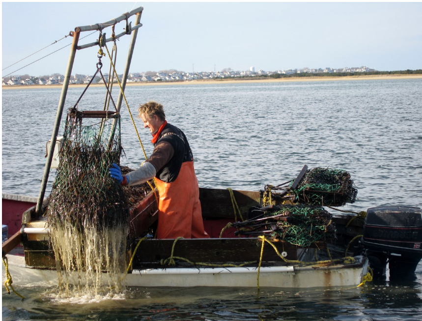
Figure 76.—Using the hoist to retrieve a bay scallop dredge in Nantucket Harbor, 2006.
