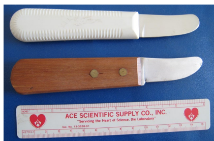
Figure 50.—The bay scallop knife has a 2-inch (5-cm) blade. The knives used for many years had wooden handles (lower), but, later, state health departments decreed that the handles had to be plastic (upper) for public health reasons.
