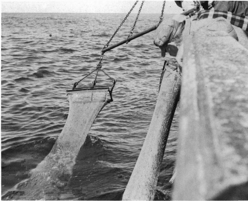
A pair of Digby dredges on a bridle, fine mesh nets streaming behind, is hauled to the forward port gallows of the R/V Albatross III during a benthic research cruise in the middle 1950's.
