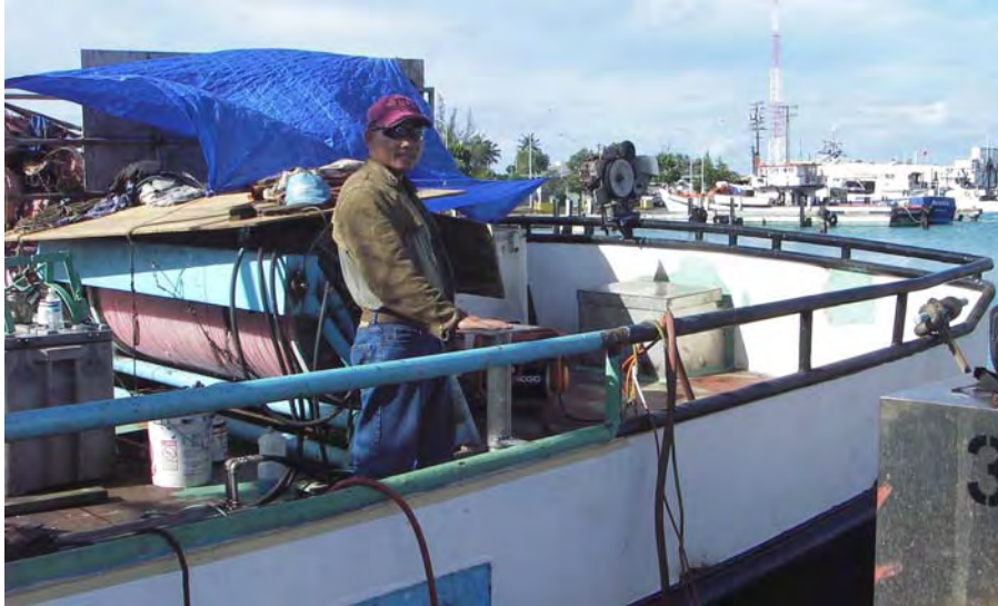
Fig. 44. F/V Seven Star II with the main line shooter mounted in its previous position in the center of the stern and welder Phon Do with his hand positioned on the new main line shooter mount located on the port side.
