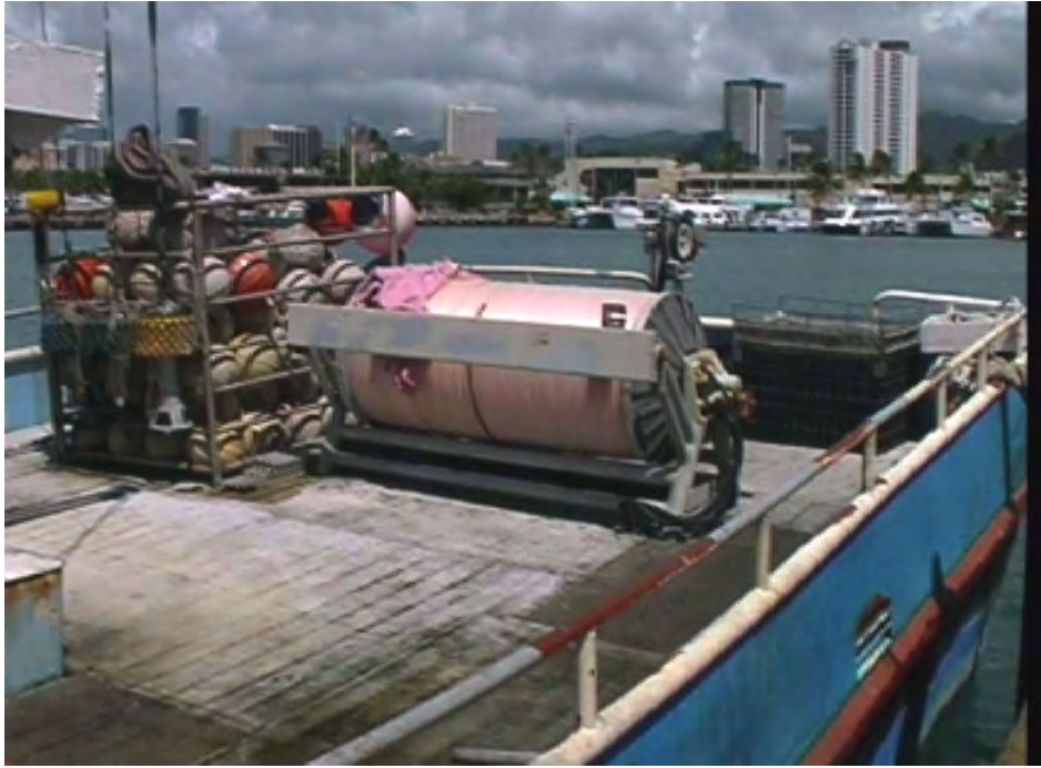
Fig. 38. F/V/ Hokuao with the main line shooter in the original stern position.
