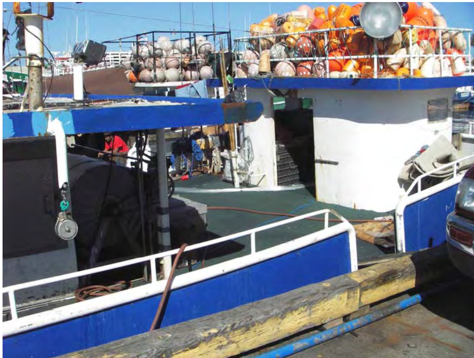
Fig. 47. F/V Crystal port-side, showing location of spool behind the cabin, setting shack, and buoy rack.
