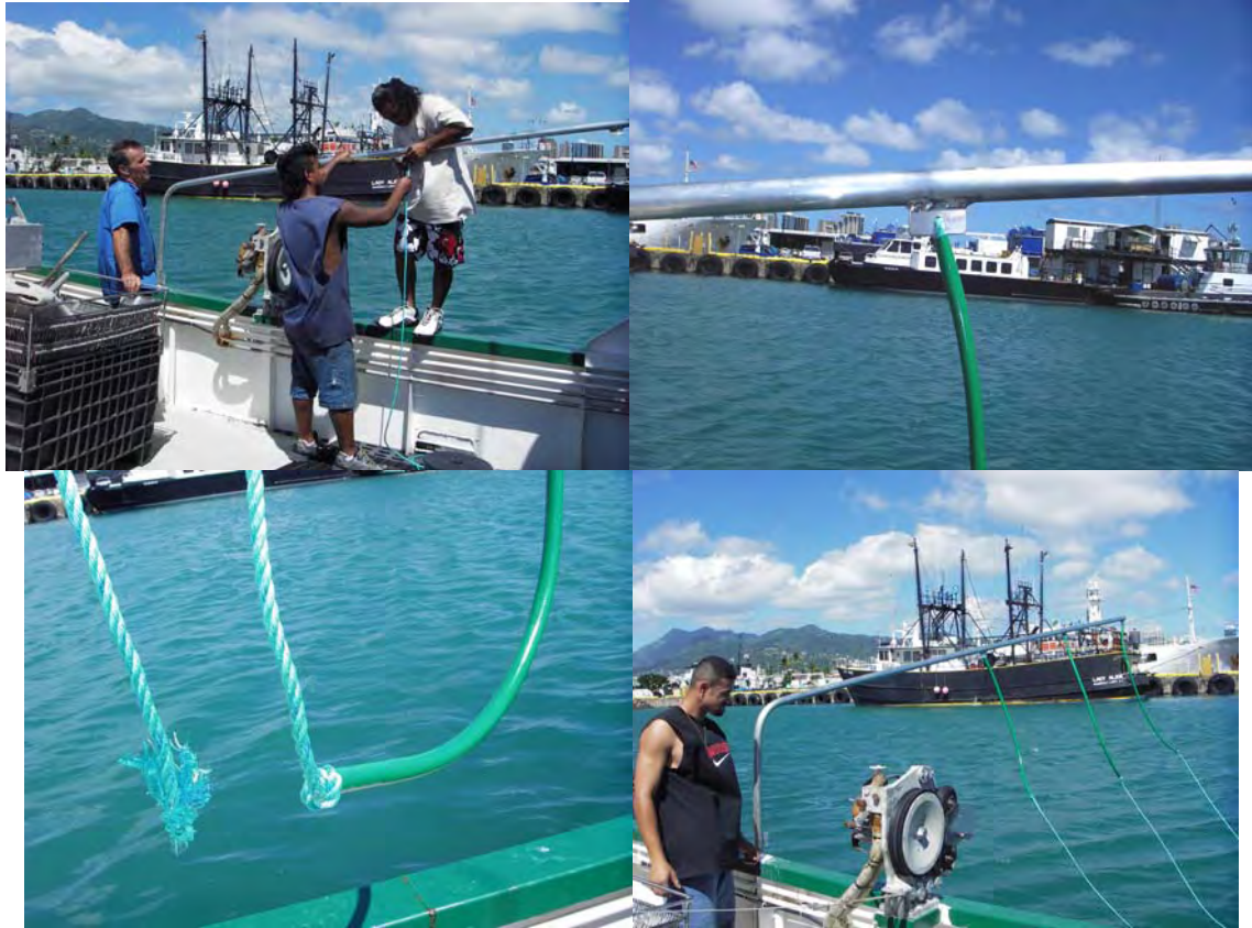
Fig. 57. Installing a bird curtain: attaching the streamers to the pole by either eye splicing through the 13 mm hole in aluminum tab on pole or onto stainless steel clips (top left), attachment of streamer to pole (top right), knot holding hose in position and either backsplice or heat seal at the end of the streamer (bottom left), and complete deployed bird curtain (bottom right).
