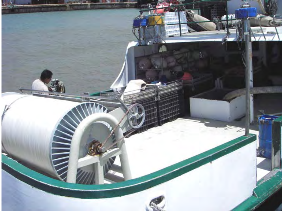
Fig. 5. F/V Finback with side-setting deck layout.
