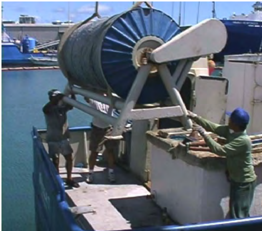
Fig. 34. Movement of the main line spool to its new position at the stern on the F/V Isabella T.
