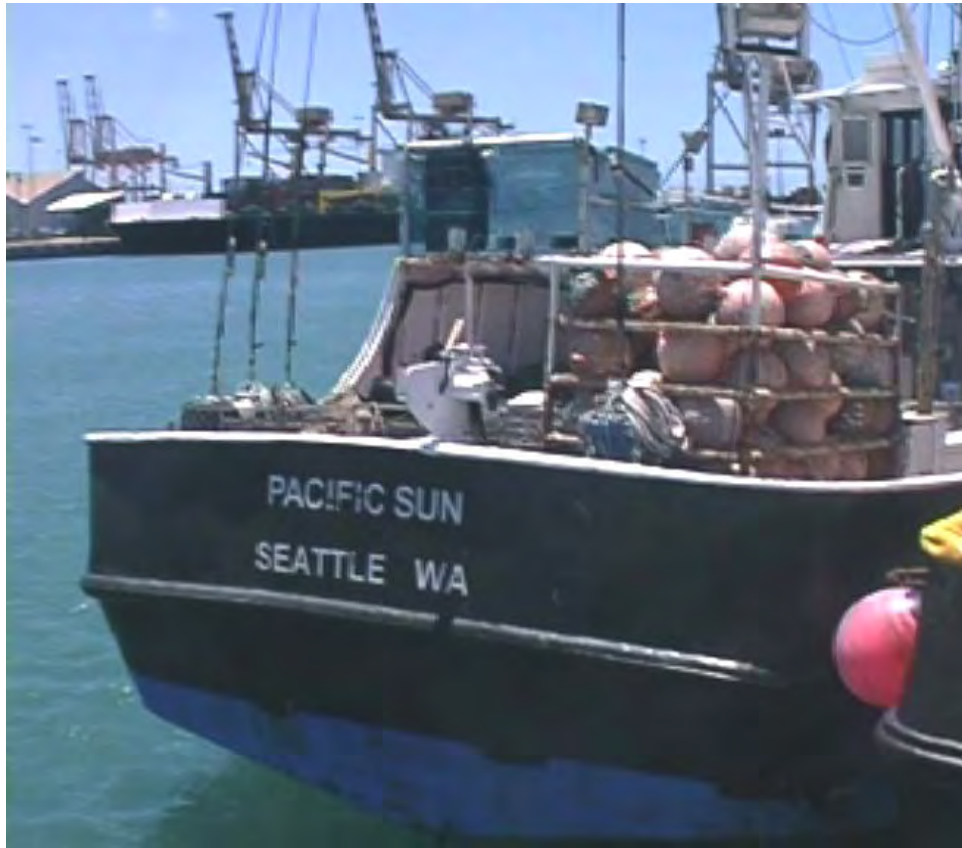
Fig. 17. F/V Pacific Sun with stern setting deck design.
