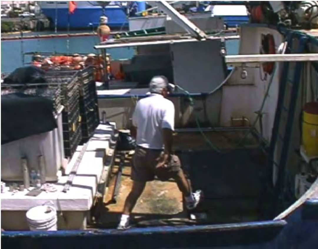
Fig. 35. F/V Isabella T deck space opened-up after movement of the main line spool to the stern.
