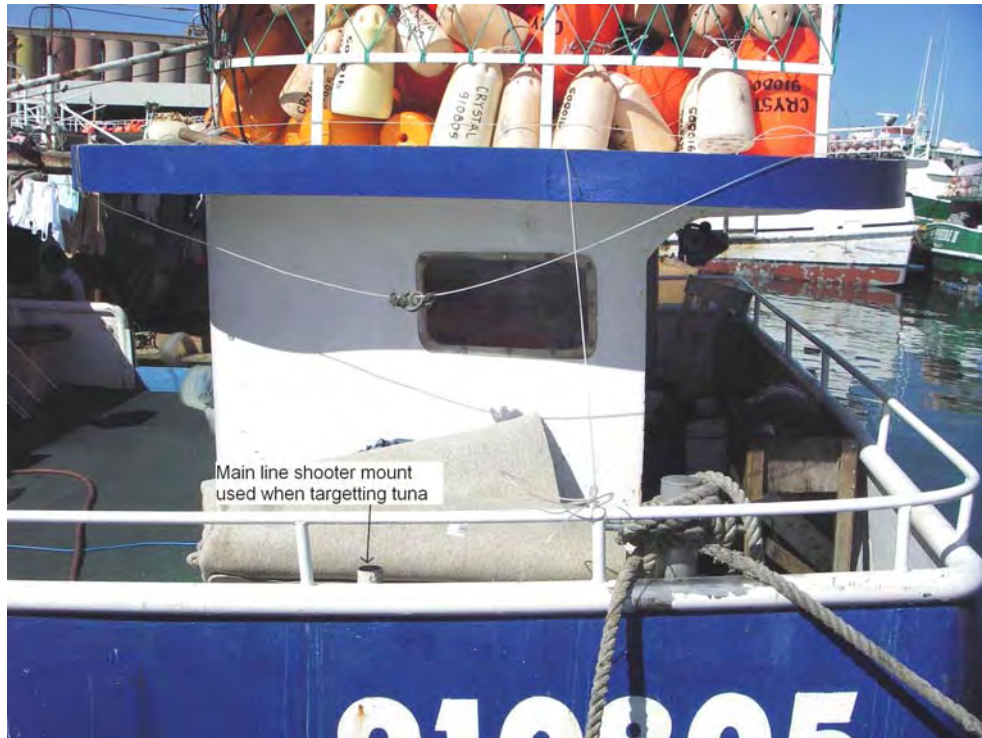
Fig. 48. Port-side main line shooter mount to be used on the F/V Crystal when targeting tuna.
