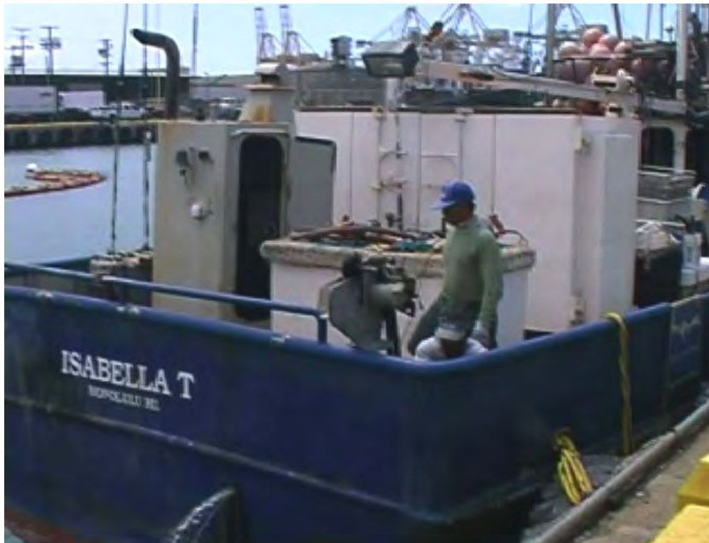
Fig. 32. F/V Isabella T before deck design changes, with the main line shooter located on the stern near the starboard side.
