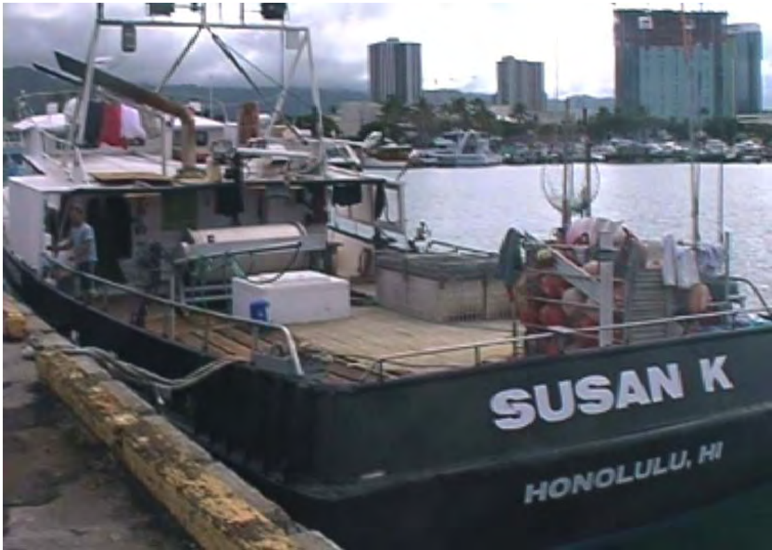
Fig. 23. Deck layout of the F/V Susan K after moving the main line shooter from the stern to the port side.
