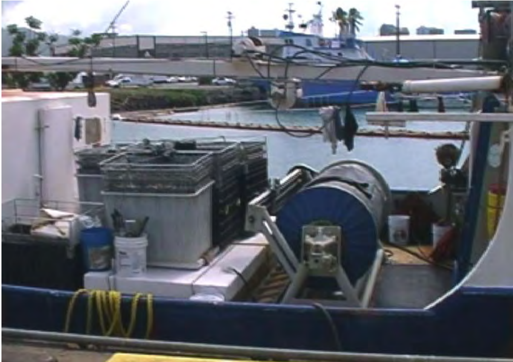
Fig. 33. Location of the main line spool on the F/V Isabella T prior to deck design changes to set from the side.
