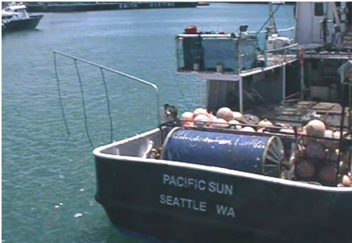
Fig. 18. F/V Pacific Sun deck design for side setting from the port side with bird curtain in deployed position. Low, wide buoy rack in front of the spool is conveniently located for hauling and setting.
