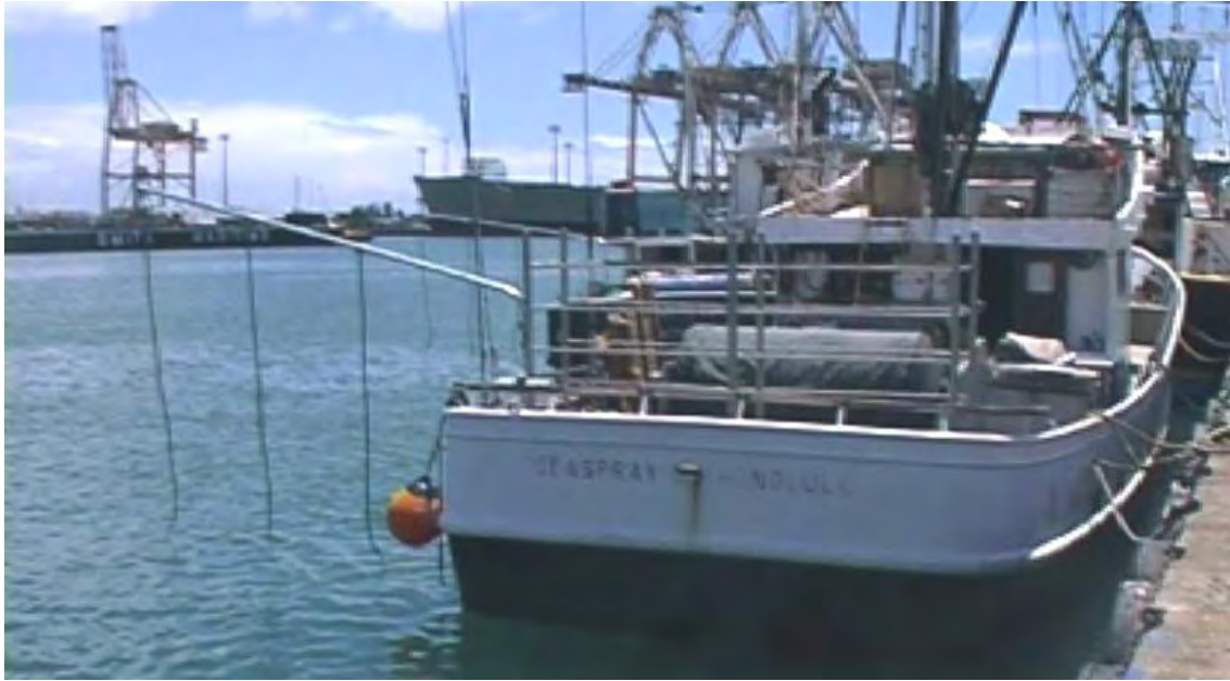
Fig. 14. Bird curtain deployed on the F/V Seaspray with converted deck.
