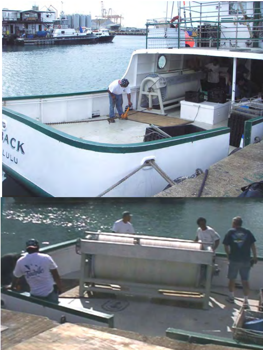
Fig. 4. Two “endless chains” used on the F/V Finback to slide the spool along the deck from the portside to the stern.
