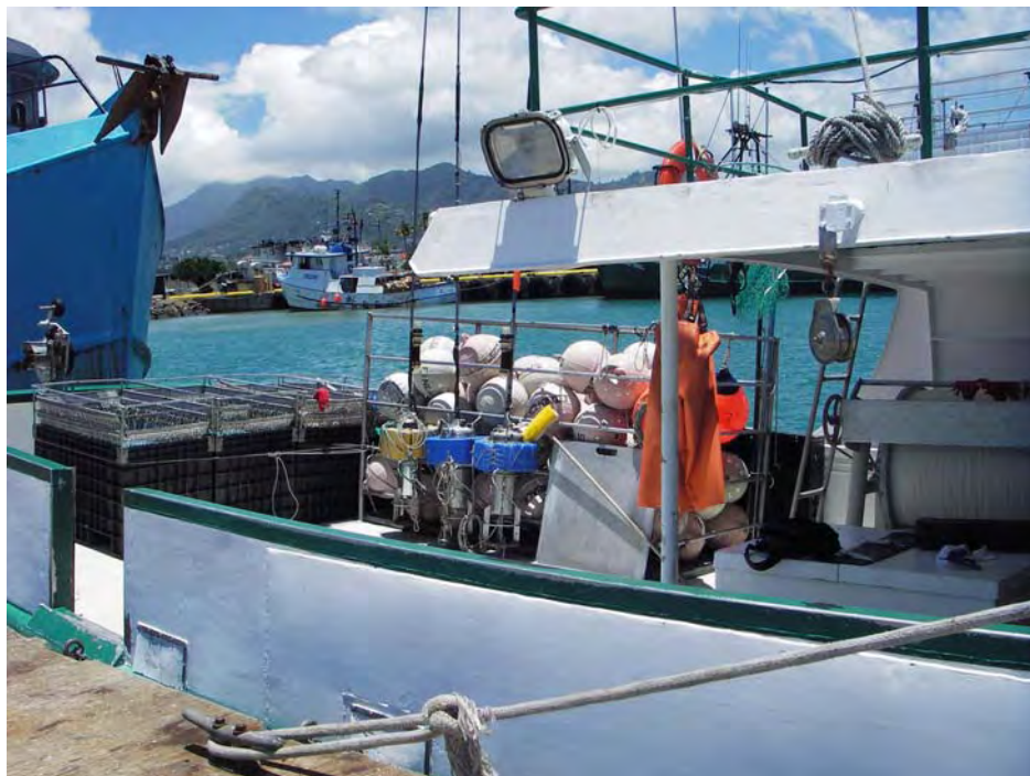
Fig. 3. F/V Finback with stern-setting deck layout.
